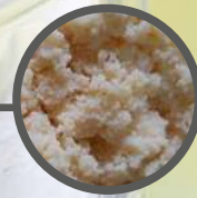
ION EXCHANGE RESIN FOR PFAS REDUCTION
